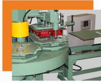
Automated tile carrier unit for quicker cycle times
